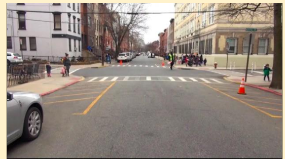
Figure 3-7. Example of Daylighting
