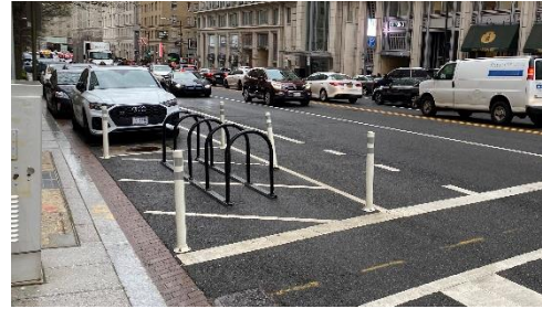
Figure 3-18. Bike Corral in Space Vacated Due to Daylighting
